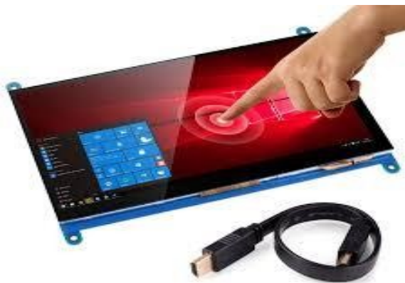
Fig: 3 shows the touch screen which will be used by the passenger.
